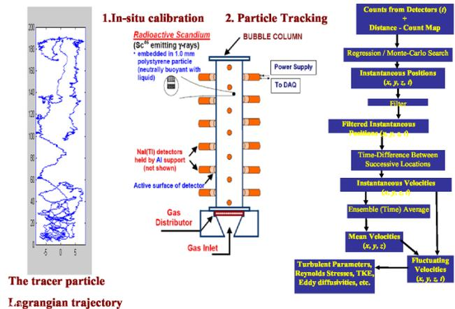
Figure 4: Lagrangian Trajectory and Data Processing Steps of RPT Technique
