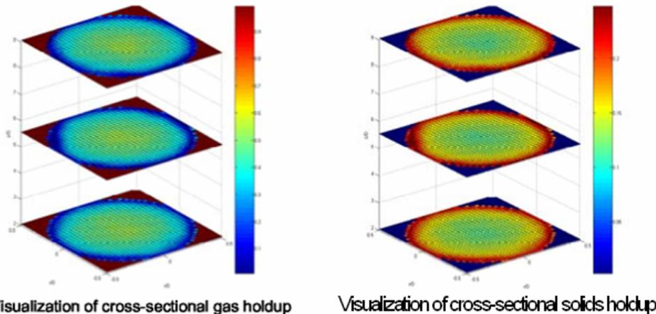
Figure 6: Example of Results of Gas and Solids Hold-up Cross Sectional Distributions along the Slurry Bubble Column Height Using CT Technique
