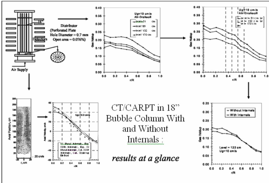
Figure 9: Flow Structure of Bubble column with and without Heat Exchanging Internals Obtained by RPT and CT Techniques.
