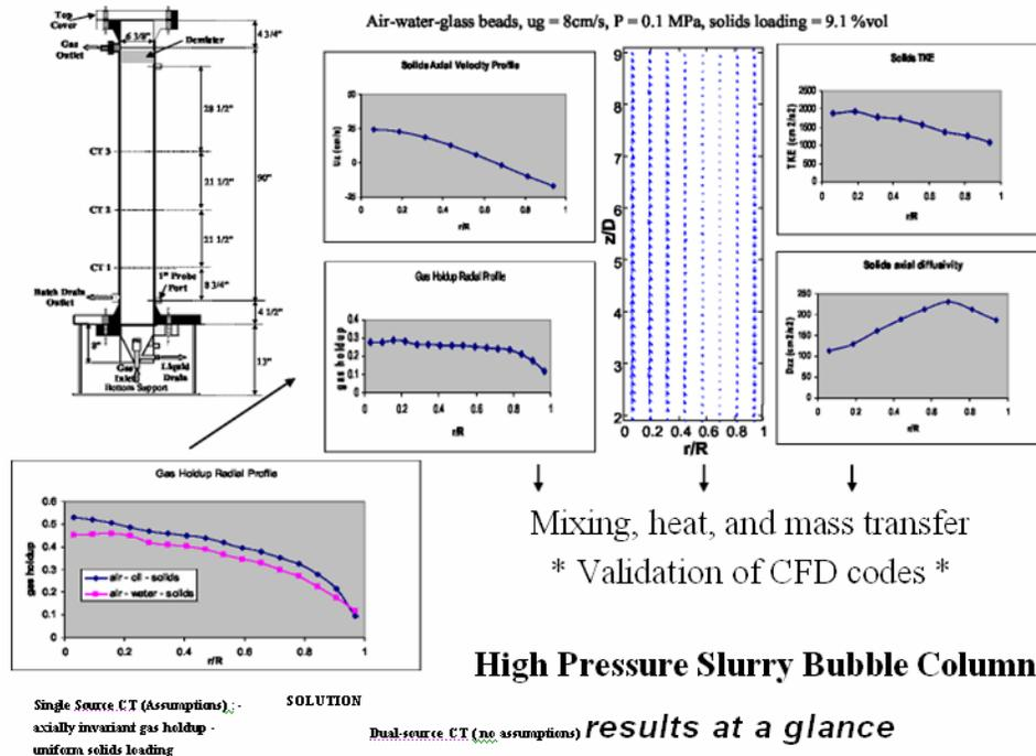
Figure 8: Flow Structure of Slurry Bubble Column obtained by RPT and CT Techniques
