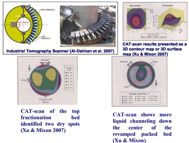
Figure 2: Industrial Tomography Scanner (ITS) and Its Application in A Pilot Plant and Commercial Scales Units
