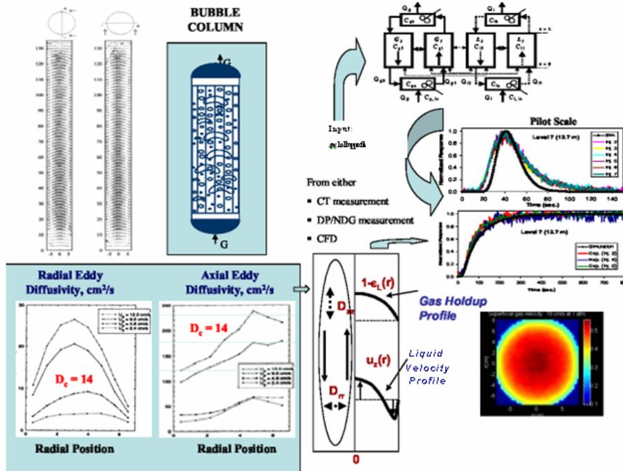
Figure 10: Integrating the Results of Radioactive tracer RTD, Densitometry, CT and RPT Techniques to Advance the Design of Bubble and Slurry Bubble Column for Methanol Synthesis from Syngas (Laporte, Texas, Alternative Fuels Development Unit).
