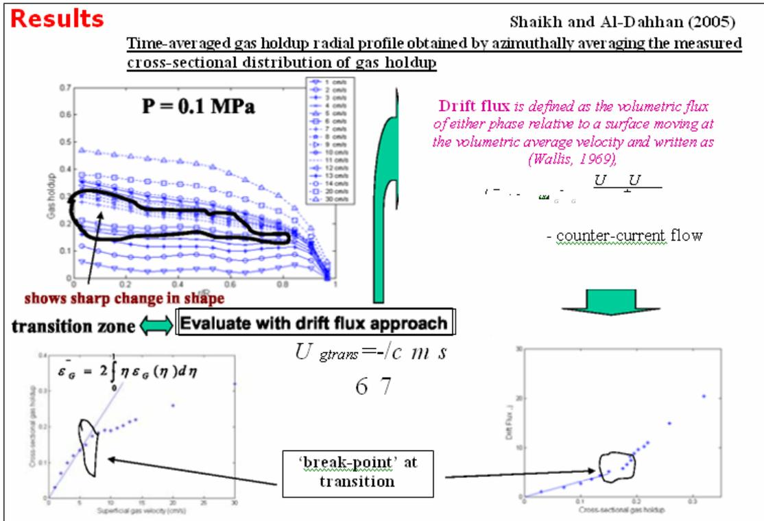
Figure 7: Identification of Flow Regime Transition in Bubble Column using CT technique
