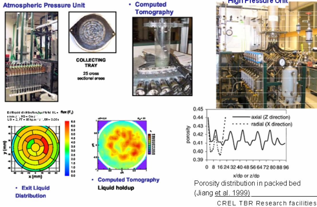
Figure 11: Example Of CT Technique Results in a Trickle-Bed Reactor and their Comparison with the Liquid Flux Collected at the Bottom.
