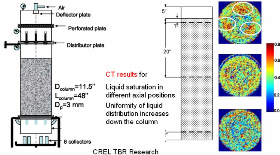
Figure 12: CT Technique application to Study the Distributor Design in a Pilot Plant Scale Trickle-Bed Reactor
