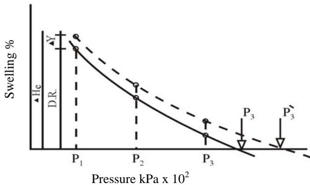
Figure 5. Effect of oedometer deformability on the measured swelling pressure using (different pressures method).
