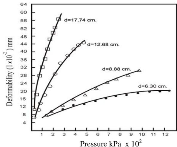
Figure 3. Deformability of apparatus for different steel disk diameters (steel disk thickness = 30 mm).
