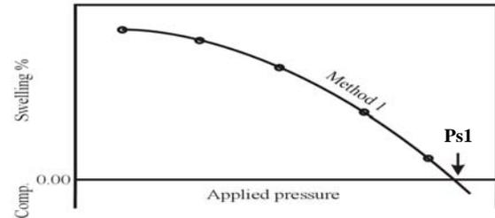
Figure 1. Determination of swelling pressure (method 1).
