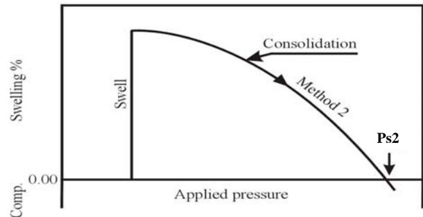
Figure 2. Determination of swelling pressure (method 2).
