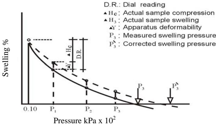
Figure 4. Effect of oedometer deformability on the measured swelling pressure using (preswelled sample method).
